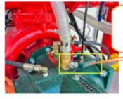
Vacuum Pump Water Valve: HORIZONTAL: Valve closed VERTICAL: Valve open
